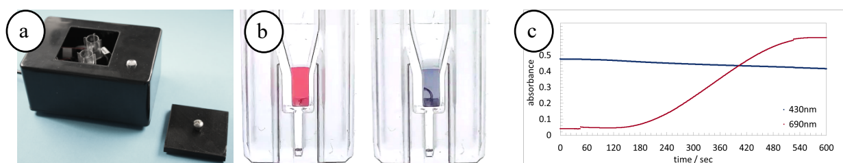
Figure 1: (a) 2-LED- \mu Spectrophotometer using two wavelengths and standard UVVIS-cuvettes. (b) Selection of colloidal AuNP solution samples containing positive isothermal DNA amplification reaction (red), negative control (blue) and MgCl_2 . (c) Corresponding absorbance measurements.
