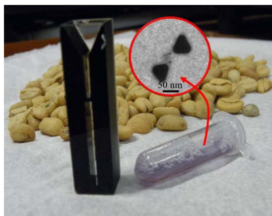
Figure 1: Image of gold nanoprisms aptasensors in suspension used in the screening test.
