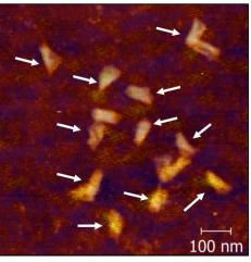
Fig. 2: iTERS image (height + diode signal) from Origamis on glass. Yellow areas Origamis with active tip. Signal loss was at half-finished image.
