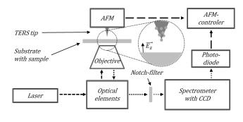
Fig. 1: schematic from the experimental iTERS setup
